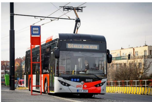
Figure 13: In-Motion Charging Trolleybus in Prague Copyright: © DPP
