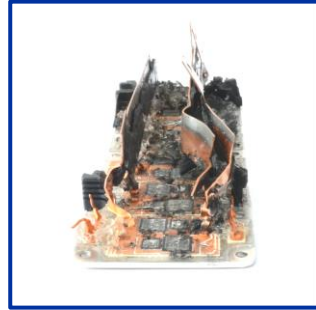
The explosive consequences of Power Semiconductor Failures (e.g., before and after the failure of a power semiconductor) [5]
