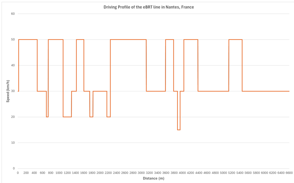
Figure 6. Route speed limits along the eBRT line in Nantes, France.
