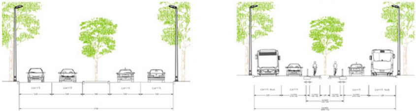
Figure 1: Reconfiguration of a section of Passeig dels Països Catalans; on the left, previous situation, on the right, the new one.
